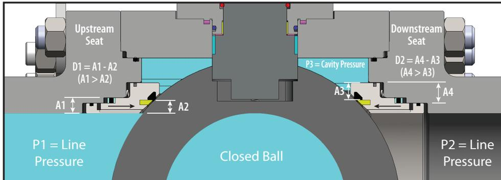
**Double Isolation and Bleed Design (DIB-1)** is the standard configuration of all **C&C Trident Series DPE** valves. This design features double piston effect seats on both the upstream and downstream sides of the valve, which, in the closed position, provides double isolation from pressure at both ends.
