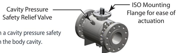
**C&C Trident Series DPE DIB-1** valves come standard with a cavity pressure safety relief valve to prevent any overpressure of fluids trapped in the body cavity.
